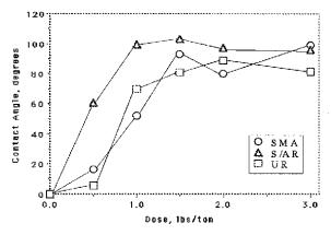
Figure 5. Dependence of Contact Angle at  $60^{\circ}$  on Surface Treatment.
