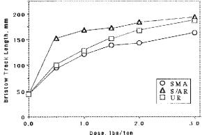
Figure 3. Dependence of Bristow Track Length on Surface Treatment.
